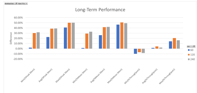
Figure 12: Long-Term Performance: the range and average value of the percentage of memory reduction and throughput improvement compared with the baseline Redis for large data size.
