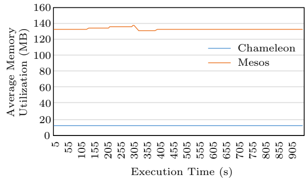
Fig.18. Average memory utilization when eight workloads co-run on the 16-node ADOM cluster over the execution time period.
